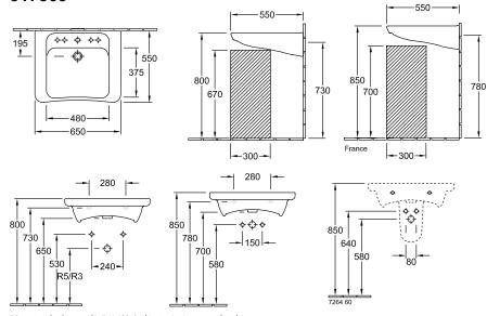
R3 Installation in acc, with DIN 18040 with standard space saving siphon R5 Installation in acc. with DIN 18040 with standard concealed siphon
